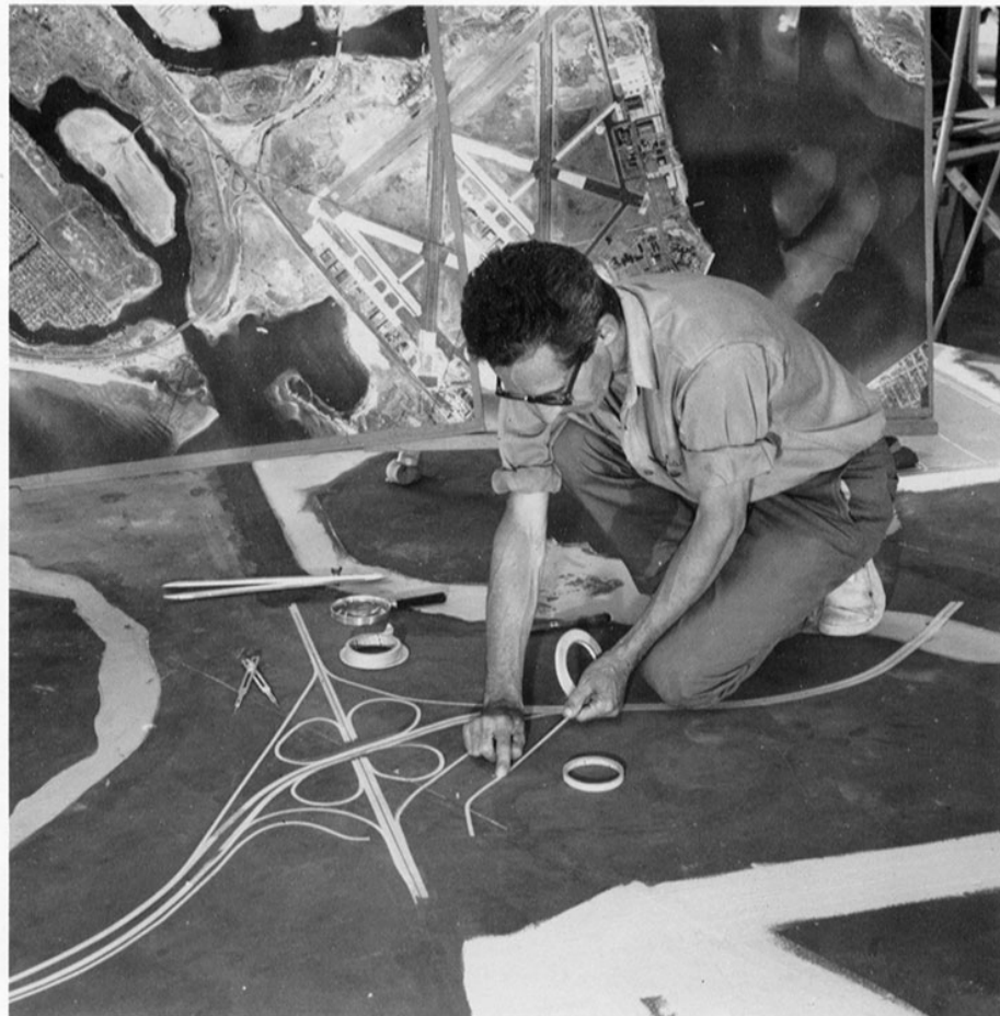
Worker applying masking tape guides before painting the roadways on the Panorama, 1963.
